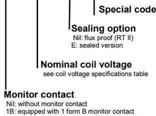
Note: For Ag plating contact (main load), add P after date code.
